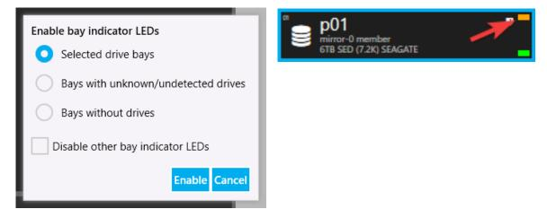
Drives with their indicating LEDs enabled will have a blinking orange indicator on Rack View as well as on the physical drive on the appliance.
